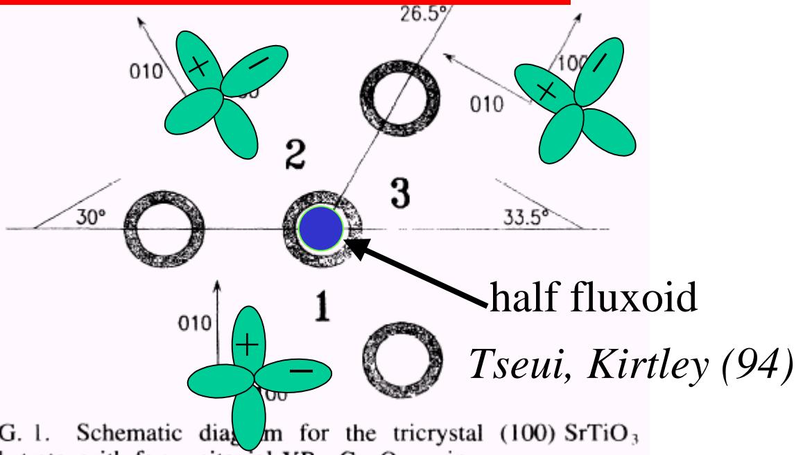
FIG. 1. Schematic diagram for the tricrystal  $(100)$   $\text{SrTiO}_3$  substrate, with four epitaxial  $\text{YBa}_2\text{Cu}_3\text{O}_{7-\delta}$  rings.
