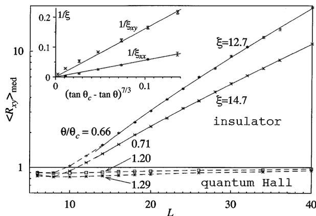
FIG. 2. QH to insulator transition in finite-size scaling. Solid lines are the best fits of Eq. (8), and dashed lines are guides to the eye. Inset: The resulting inverse correlation lengths are consistent with the critical exponent  $\nu = 7/3$ .
