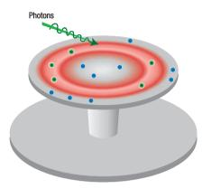
Figure 1 Semiconductor quantum dots in a disk microcavity. The photonic modes of the cavity (red) are concentrated in proximity of the disk circumference. Those quantum dots (green) located within the cavity modes can be 'written' or 'read' by photons.
