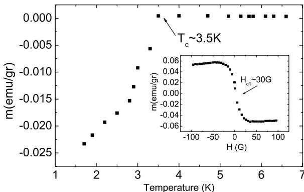
FIG. 1. Magnetization measurements of the  $\text{Na}_x\text{CoO}_2 \cdot y\text{H}_2\text{O}$  vs temperature. The transition temperature is 3.5 K. Inset:  $M$  vs  $H$  for the same sample.  $H_{c1} \sim 30$  G.
