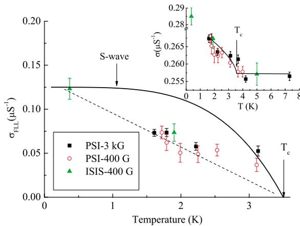
FIG. 3 (color online). The part of the muon relaxation associated with the flux lattice formation  $\sigma_{\text{FLL}}$  as a function of temperature. The solid line is the temperature dependence predicted by the two-fluid model and an S-wave gap. The dashed line is a guide to the eye. Inset: The total muon relaxation rate, as taken in ISIS and PSI in a field of 400 G and 3 kG.
