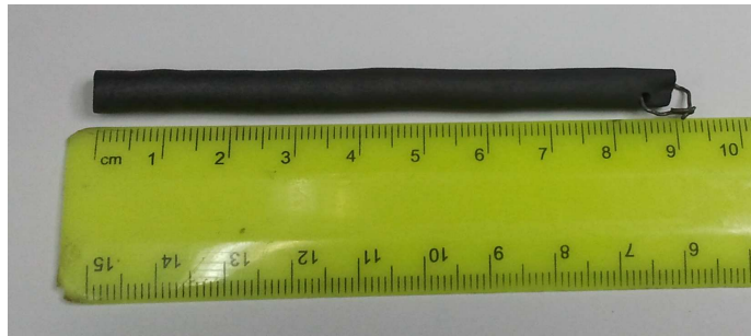
FIGURE 2.3: A sintered feed rod of LSCO.
