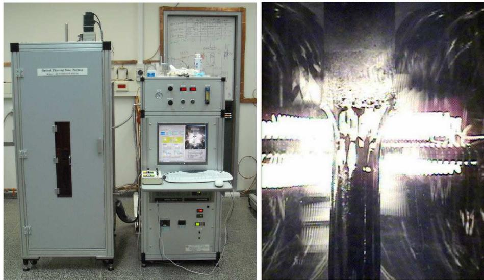
FIGURE 1.9: **LSCO single crystal during growth.** Left: The floating zone furnace at work. Right: Feed and seed rods are connected with a molten zone in between during crystal growth.
