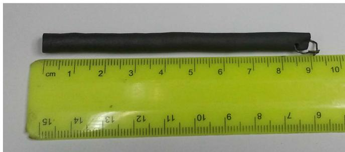
FIGURE 1.10: A sintered feed rod of LSCO.
