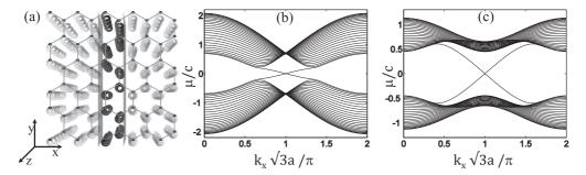
FIG. 1. (a) Honeycomb lattice, made from helical waveguides. The black waveguides between the two lines represent a unit cell in the x direction. (b) Spectrum of eigenmodes (in units of the coupling constant) for a finite lattice in the y direction, with  $A_0 = 2$  and  $\Omega = 10c$ . (c) Same as (b), but with  $A_0 = 3$  and  $\Omega = 3c$ .
