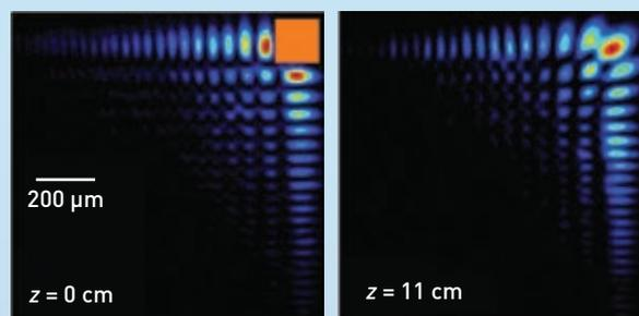
Self-healing is easiest to understand in terms of a ray picture; the main spot of the accelerating beam is described as a bundle of rays forming an envelope near the intensity maximum.
