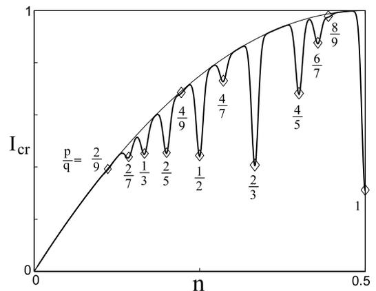
FIG. 3. Schematic diagram of critical currents versus Cooper pair density  $n$  for an array of size  $L_x = 20$  and  $L_y = 2$ . Rational numbers  $p/q = n_q L_y$ , which label the dips at  $n_q$ , are indicated. The classical critical current is depicted by a thin line. Above the critical currents at  $n_q$ , fractional ac Josephson frequencies are expected at  $2eV/hq$ . Spatial disorder and finite temperature are introduced qualitatively by broadening of the dips.
