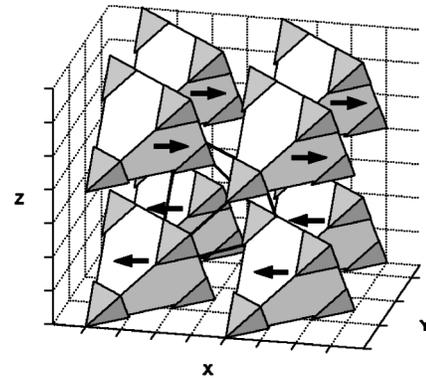
FIG. 3. The pyrochlore viewed as a cubic lattice of supertetrahedra. The arrows show the direction of the supertetrahedra's pseudospin in the mean field ground state.
