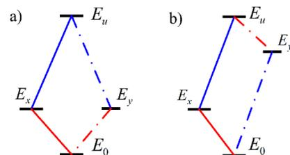
FIG. 1 (color online). Two alternative level schemes that can be used to generate entangled pairs. The solid (dashed-dotted) line represents the decay channel that yields two  $x$  ( $y$ ) polarized photons. The energies correspond to the colors of the emitted photons. (a) Represents the situation where photon colors match in the first generation, and has the geometry of a kite (deltoid). (b) Represents the case where colors in different generations match, and is geometrically a parallelogram.
