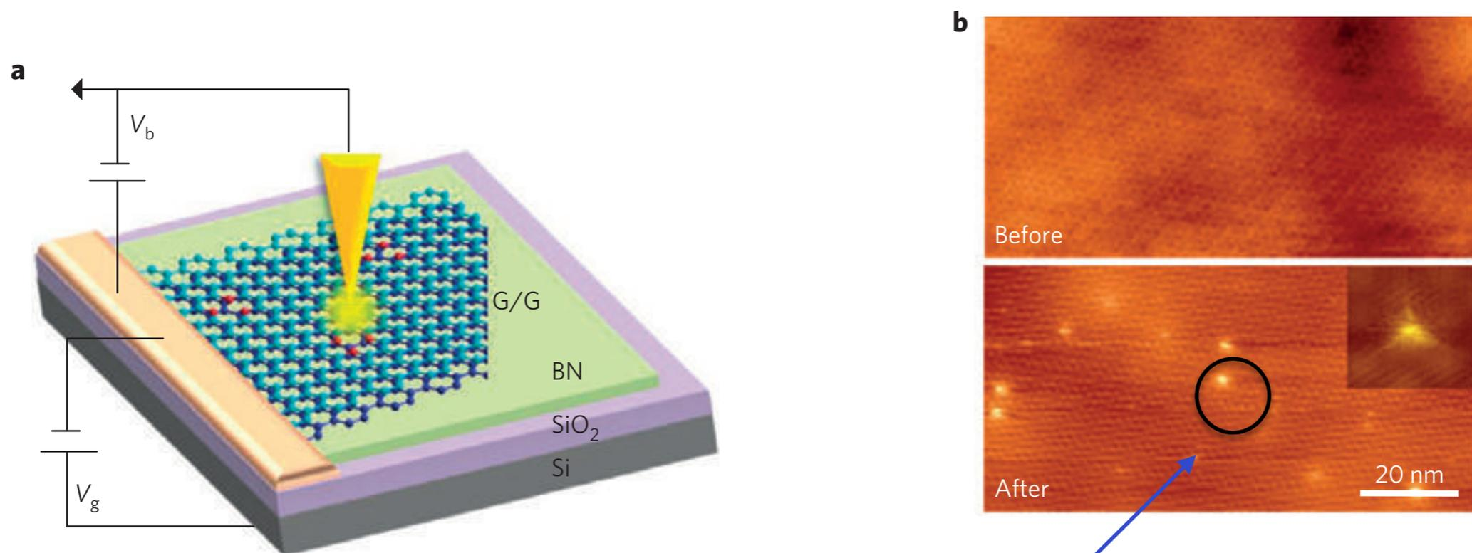
Local vacancy. Local charge is changed by applying voltage pulses with the tip of an STM
