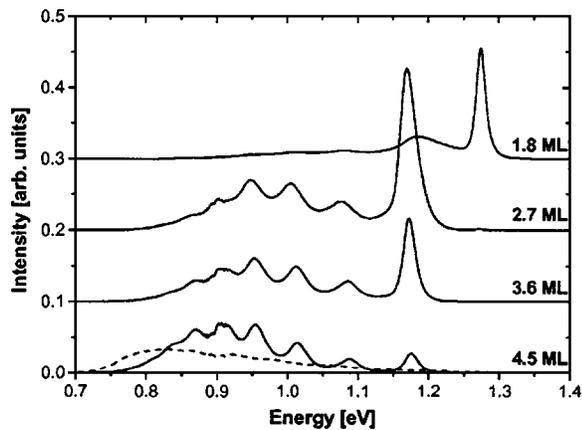
FIG. 4. 77 K PL spectra of nominally 1.8 to 4.5 ML  $\text{Ga}_{0.18}\text{In}_{0.82}\text{As}$  QD layer on InP. Also shown, as a dashed line, is the 77 K PL spectrum of nominally 2.4 ML InAs QD layer on InP.
