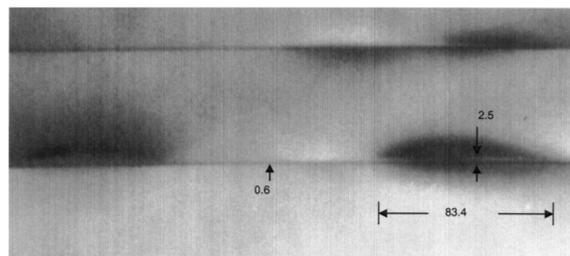
FIG. 1. TEM image of a double stack of InAs QDs grown on InP. Indicated dimensions are in nanometers.
