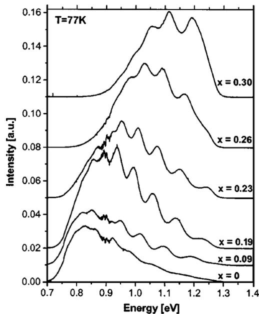
FIG. 2. 77 K PL spectra of nominally 2.4 ML InAs QDs layer on a  $\text{Ga}_x\text{In}_{1-x}\text{P}$  layer for gallium content ranging from  $x=0$  to  $x=0.3$ .
