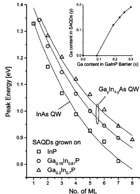
FIG. 3. Measured (symbols) and calculated (lines) QD PL emission energies at  $T=1.8$  K. The inset shows the fitted gallium content in the QDs ( $y$ ) as a function of the gallium content in the GaInP layer ( $x$ ).
