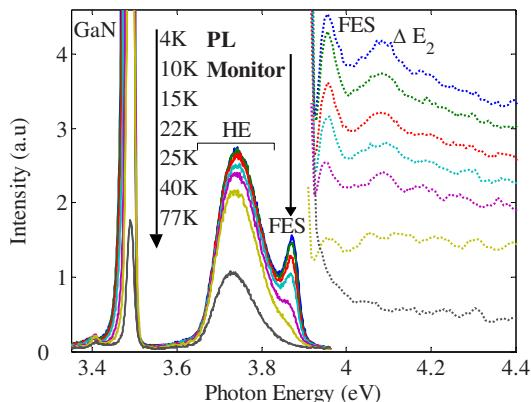
FIG. 2. (Color online) PL (solid lines) and PLE (dotted lines) spectra of sample A for various temperatures. GaN, HE, and FES refer to the spectral features discussed in the text. The PL was monitored at the FES peak.
