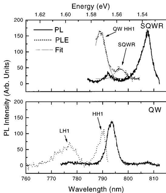
FIG. 3. Near-field PL (solid line) and PLE (dotted line) spectra of the 80 Å (110) QW (lower panel) and the 150 Å × 80 Å SQWR (upper panel). A two Gaussians model fit used to determine the relative intensity is shown by the thin solid line.
