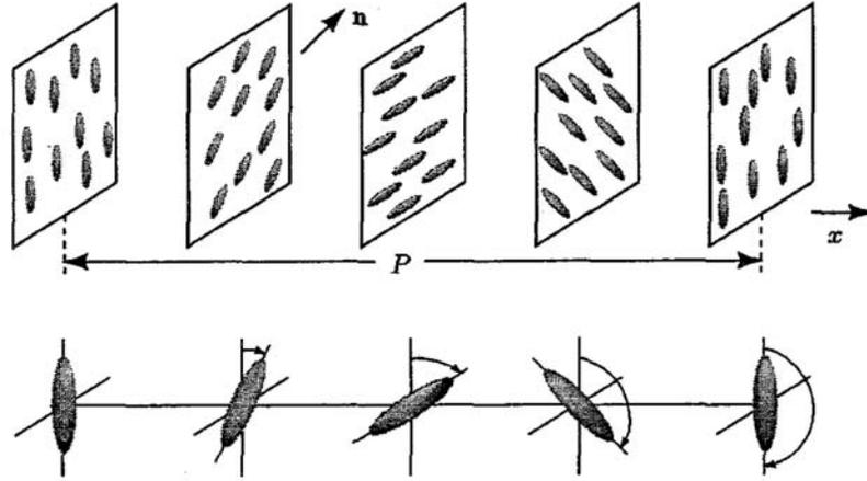
Figure 1.3: Cholesteric phase: This phase is composed of molecules which contain chirality. We see in the figure that a global chiral axis is established; this is the pitch. Along every location on the axis a perpendicular layer is established in which the molecules are aligned along a local director. The director rotates around the pitch in a helical pattern proportionally to the strength of the pitch.
