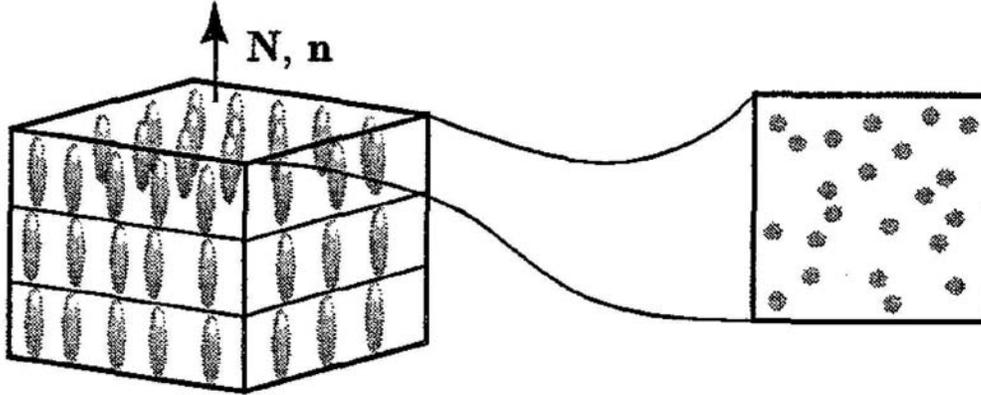
Figure 1.4: Smectic A Phase: The figure shows that the molecules in this phase are ordered in density layers. The molecules are not free to move in a three dimensional space, they are constrained to the x-y layer plane. Their axes are aligned with a director that is perpendicular to the layers plane. In the right figure a bird view is seen. It shows that in two dimensions the molecules are scattered arbitrary.
