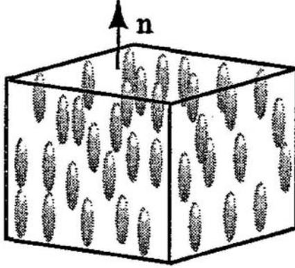
Figure 1.2: Nematic Phase: This phase is characterized by the appearance of the director. This is a unit vector in the mean direction of the molecules. The molecules in the sample deviate only slightly from this direction and are on average parallel to each other but their center of mass is still positioned arbitrarily.
