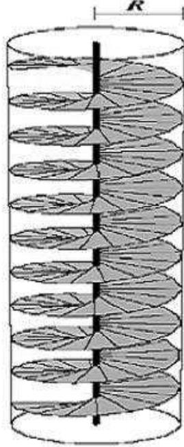
Figure 1.5: A Screw Dislocation in a layered material is a defect: It has a core around which it twists and lifts the layers in a helical pattern having the shape of a staircase. The radius of a dislocation is the radius beyond which the molecules are relaxed to their origin directions in the samples.
