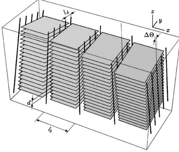
Figure 1.7: The TGB Phase in this picture follows a pitch which lies in the  $x$  axis direction. It is composed of SmA grains with inter-layer distance of  $d$ . The angle between consecutive grains of SmA is  $\Delta\Theta = 2\pi\alpha$ . The grains length is  $\ell_b$  along the pitch. Between grains an array of parallel screw dislocations reside perpendicular to the bordering layer planes. The dislocations in each array are separated by  $\ell_d$ .
