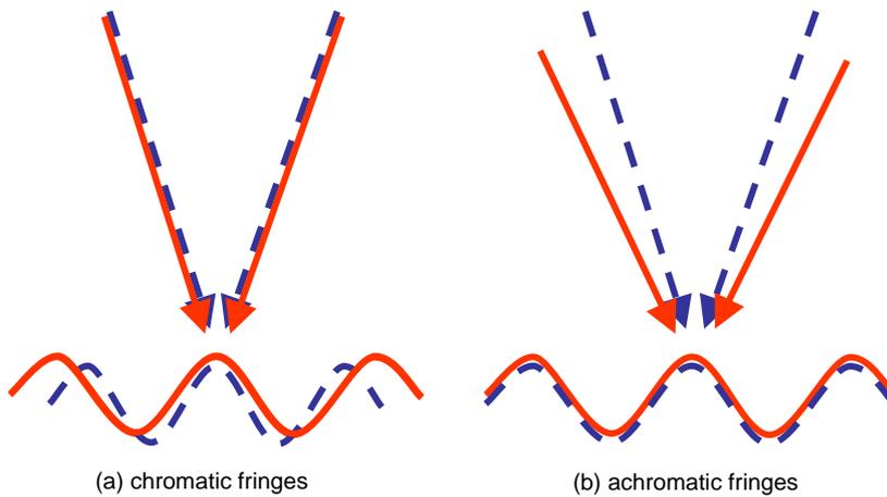
**Figure 5:** (a) When the two white-light interfering beams create fringes, the side fringes in red (full line) and blue (broken line) do not overlap and, upon addition, smear into gray. (b) When the interfering beams are magnified linearly with colour, the fringes now overlap at all colours. The colours have been shifted slightly for display purposes.
