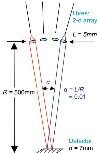
**Figure 2:** Non-redundant, two dimensional beam combination in three-dimensional space. The  $f$ -ratio of the fibres is extended by lenslets to be nearly collimated. The fibres and lenslets are inside a square of size  $L \times L$  at a large distance  $R$  from the detector. The number of monochromatic fringes is  $\approx R/L$ . Typical dimensions are given.
