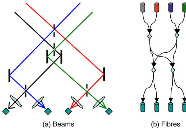
**Figure 1:** Michelson combination of (a) beams or (b) fibres using beam splitters or couplers. The Fibre option also requires accurate intensity calibration of each input, achieved with more splitters and detectors (not shown). These are essentially two-dimensional schemes.
