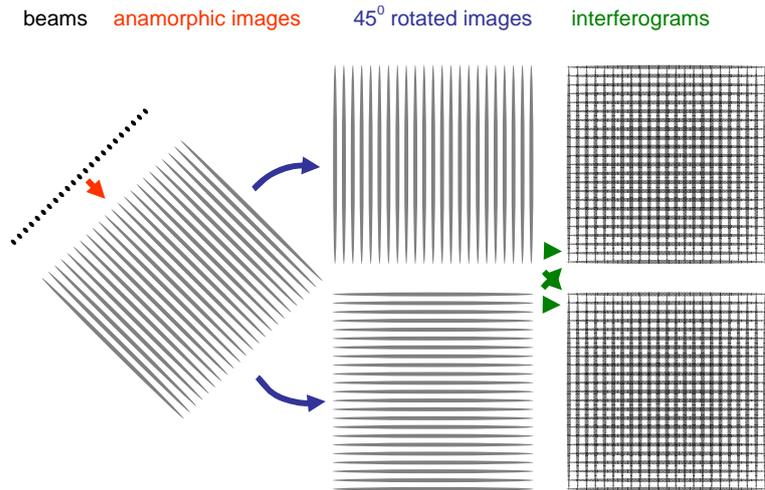
**Figure 3:** First the  $N$  beams are stretched anamorphically to  $N$  times their size. Then they are interfered with their rotated copy. As a result, we obtain white-light fringes between each beam and all the other ones.
