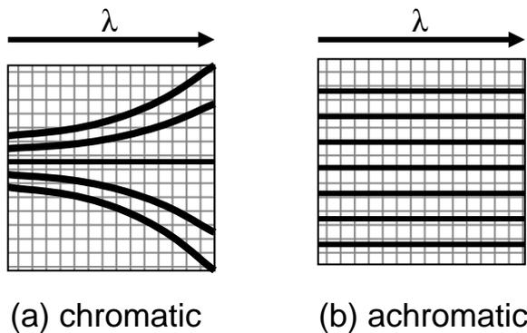
**Figure 7:** (a) Channelled spectra, chromatic fringes (only one set shown, between two beams). The fringes' spacing varies with wave length and requires more pixels and complex processing. (b) When the fringes are achromatised, the fringes become linear and make detection and calculation simpler.
