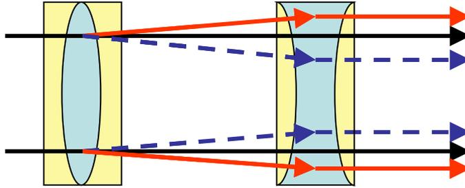
**Figure 6:** Achromatic fringes using triplets of crown-flint-crown inside parallel slabs. A ray at a wave length where the indices are equal is not deflected. A ray at shorter wave length (broken line) is deflected twice to create a narrower beam, and a ray at longer wave length is deflected twice in the opposite directions to create a wider beam. The distance between the triplets is so adjusted to get a beam width linear with wave length.
