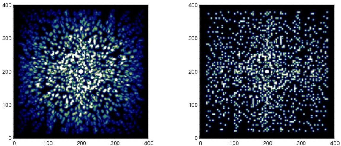
**Figure 4:** Fourier transforms of the fringe patterns between 36 beams in a non-redundant spacing (pseudo colour scale representing intensity). Even though the relative bandwidth is rather narrow (left, 620-640 nm) there is smearing of the Fourier frequencies compared to monochromatic fringes (right). Actually, the fringes on the right were achromatized to within 5% for the much wider band of 600-700
