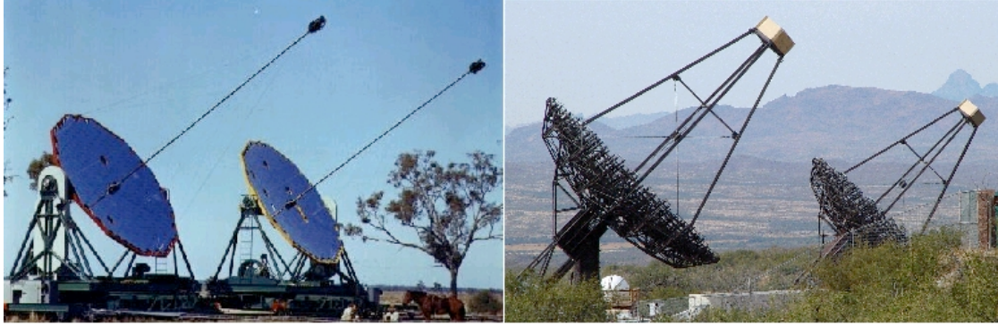
Figure 3: The two telescopes used in the Narrabri interferometer (left) have many common points with present air Cherenkov telescopes such as in VERITAS (right). The VERITAS telescopes are 12m in diameter while the Narabri telescopes were 6m in diameter.
