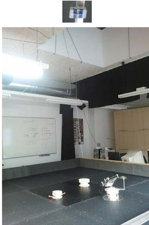
Fig. 3: Air table facility. Three nanosatellite (partial) models are placed on the table. Both “star” and radio receiver are installed ~3m above the centre of the table.
