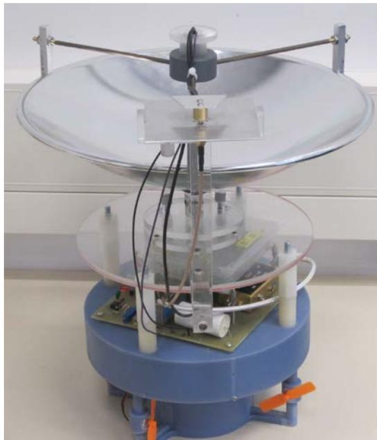
Fig. 2: Nanosatellite model. From top: photomultiplier (centre) and antenna (closer), light-collecting dish, tilt mechanism, signal preamplifier and transmitter, rotation propellers.
