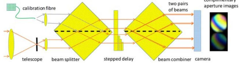
Fig. 2. The two interfering pairs of beams form fringes on the detector. Adding delays in stairs will produce many more fringes, and thus much higher spectral resolution.
