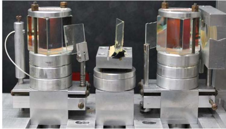
Fig. 3. Side view of the interferometer at the telescope. Thin microscope slides introduced a single delay for compensation of beam splitters path difference and misalignments [6].
