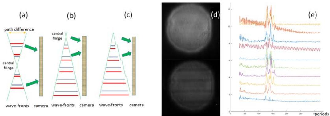
Fig. 7. (a) Two sets of colour fringes projected on the camera, the white fringe is in the centre. (b) With added delay, it is just inside the detector area. (c) One wave front has additional delays, adding more fringes and finer spectrum. (d) A xenon interferogram broken into 5 stripes (both outputs, slightly defocused). (e) The 10 stripes are inverse-transformed individually. The Xe coherent lines show even at bottom, for the longest delays ( $\sim 8\text{mm}$ ).
