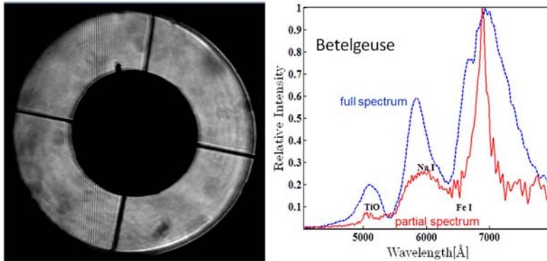
Fig. 4. (Left) Stellar fringes on 1m telescope aperture, here showing the central white-light fringe. (Right) Spectra retrieved from the entire interferogram (blue, dashed) and from the selected part of the interferogram without the central fringes (red). A significant contrast improvement is clearly seen.
