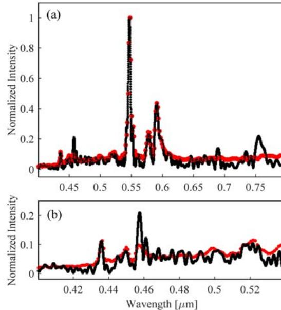
Fig. 5. (a) A metal halide lamp Fourier spectrum from a rotated (black) and vertically aligned (red) interferogram. (b) High frequency (short wavelength) part of the spectrum in (a) showing more delicate spectral features for the rotated fringes.
