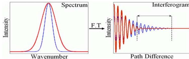
Fig. 1. Fourier band-pass filtering of the spectrum. (Left) Two spectral features with different widths. (Right) The interferograms of both spectral features with the chosen delay range bring out the sharper narrow feature, and reduce high-frequency noise.
