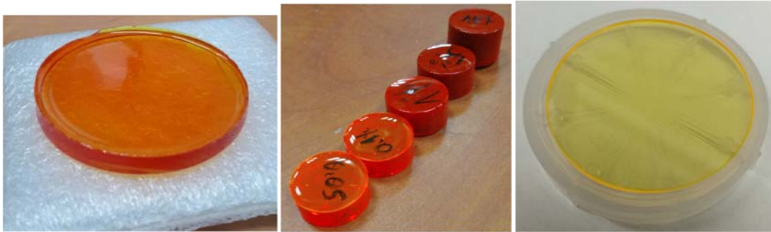
Fig 4: From left: DCM:PMMA fabricated in our lab and polished by Shamir-Eyal Ltd; DCM:CR7 fabricated by Shamir-Eyal Ltd; PMN:PMMA top layer fabricated at the Austrian Institute of Technology.
