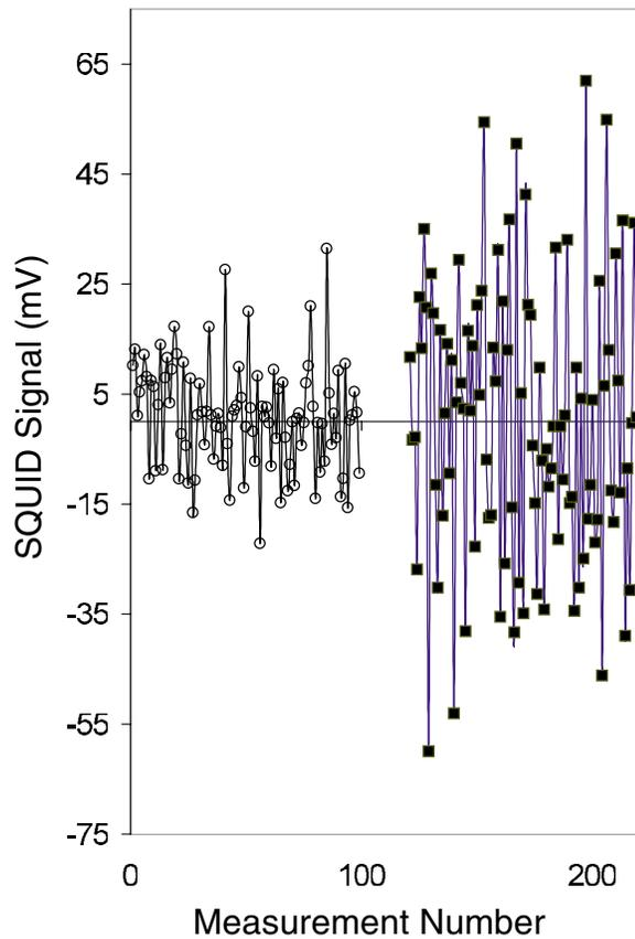
FIG. 2 (color online). Typical sequence of 100 raw data readings of the magnetometer, each following a separate quench at a rate of  $10^8$  K/s. Open symbols: control sample (“noise”); solid symbols: superconducting film. The conversion into flux units is  $4 \text{ mV}/\phi_0$  for the noise and  $1 \text{ mV}/\phi_0$  for the signal from the superconducting film. The lines connect successive data points.
