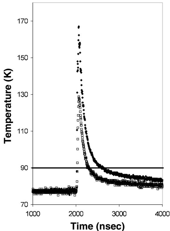
FIG. 1. Temperature cycle of the film after a laser pulse. The energy of the pulse is 7.1 mJ (solid symbols) and 3.1 mJ (open symbols). The horizontal line is  $T_c$  for our sample. Note that the cooling rate through  $T_c$  is slower for the high energy pulse.
