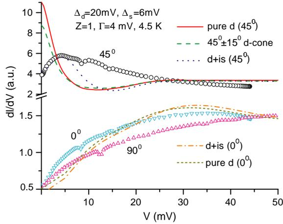
Fig. 4 – Measured conductivity (symbols) and model fitting (lines) of a few junctions.
