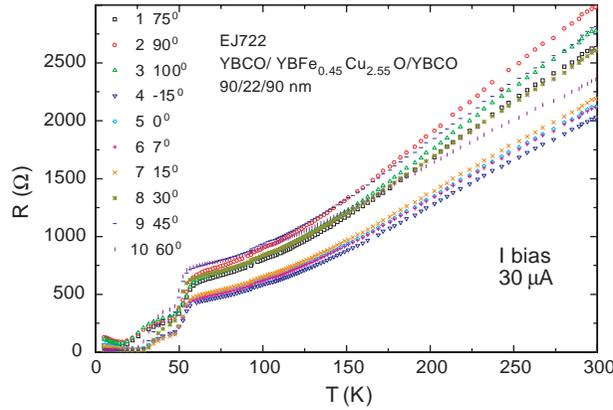
Fig. 2 – Resistance *vs.* temperature of the 10 junctions on the wafer.
