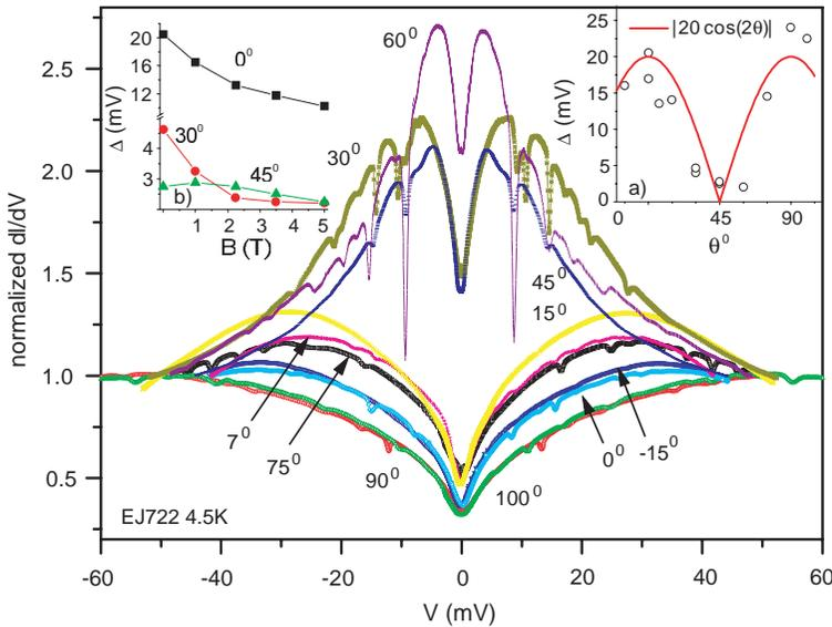
Fig. 3 – Normalized conductivity *vs.* voltage bias. Inset a) gives the angular dependence of the peak-to-peak gap parameter and inset b) the magnetic-field dependence of some gaps.
