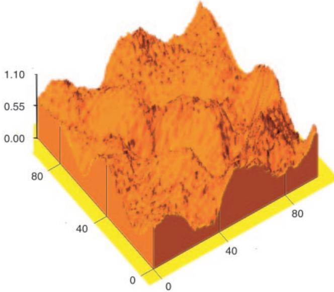
Fig. 1 – AFM image of a typical exposed ramp of an YBCO base electrode near one junction.
