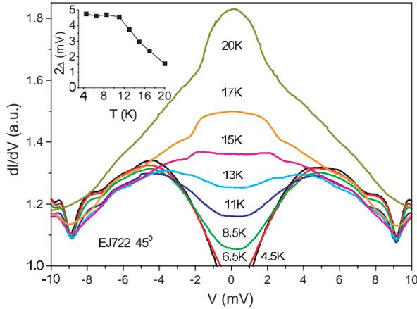
Fig. 5 – Temperature-dependent conductivity of the  $45^\circ$  junction (main panel), and the gap *vs.* temperature (inset).
