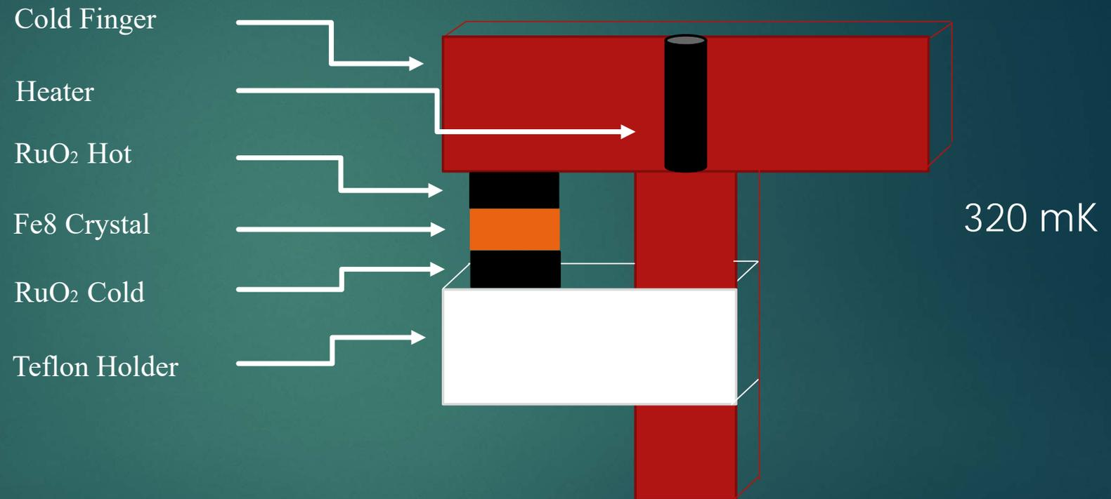
Recording the thermistors voltages after applying a voltage pulse in the heater resistor.
