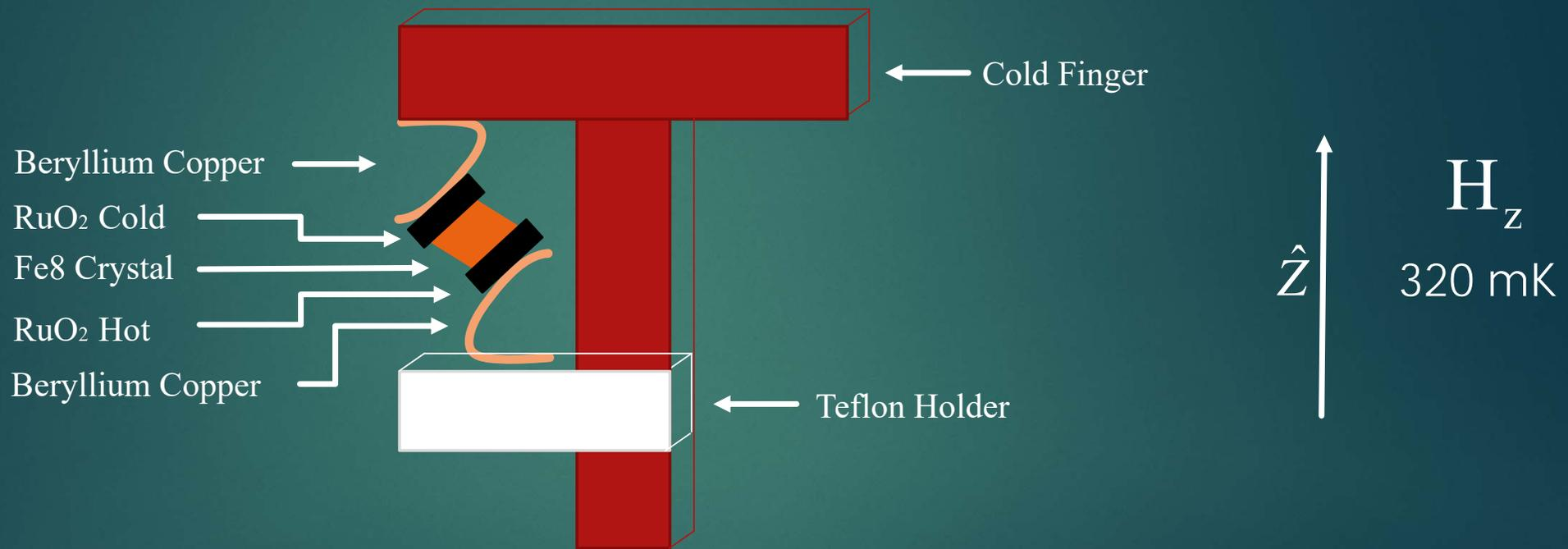
Recording the thermistors voltages while sweeping the magnetic field from +1 to -1 T.
