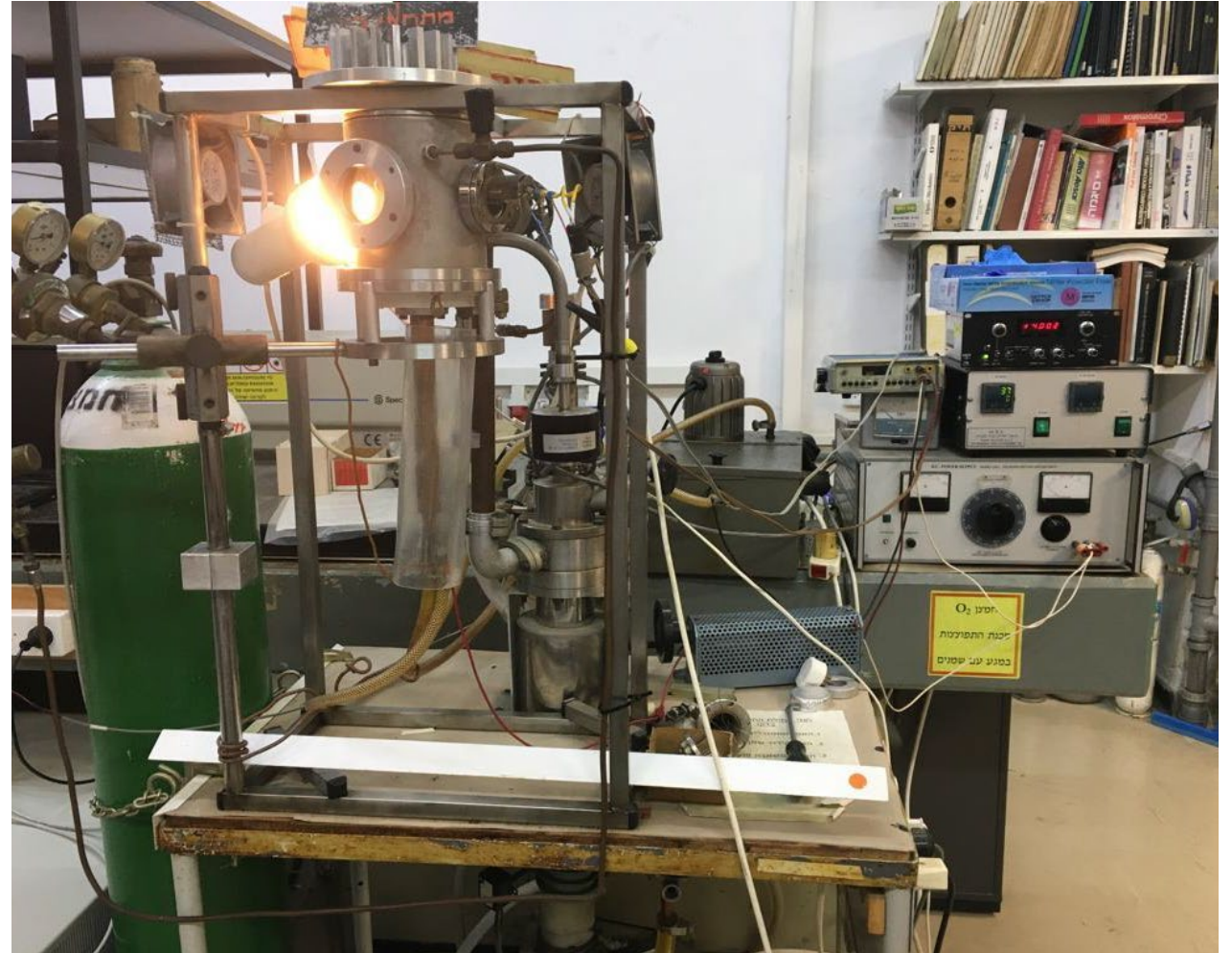
The sputtering system at Prof. Gad Koren's laboratory
