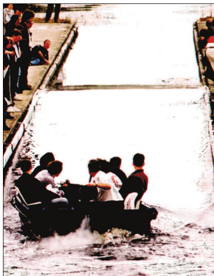
Reenactment of J.S. Russell's mid-19th century sighting of a soliton wave in a shallow water canal in Scotland. The single isolated water wave traveling in front of the boat is the soliton. Without the nonlinear action, an isolated water wave would broaden within a very short propagation distance. Here the boat generated the wave, which became an independent entity: a soliton.
