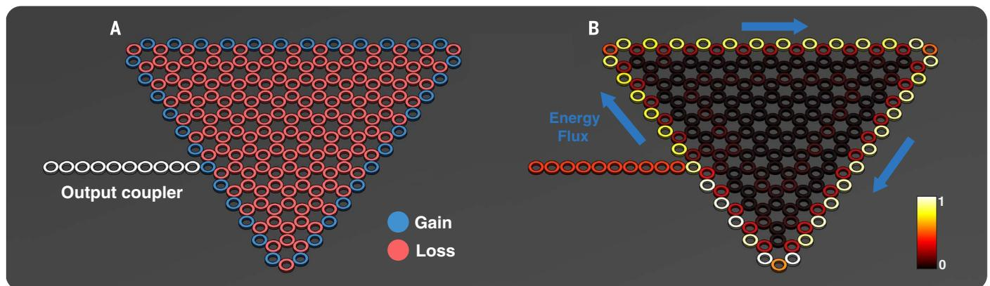
**Fig. 1. Geometry and lasing mode in a topological insulator laser based on the Haldane model.** (A) Cavity geometry (same for topological and trivial): a planar honeycomb lattice of coupled microring resonators. The cavity has unpumped (lossy) resonators (red), pumped resonators (blue), and an output channel (white). (B) The steady-state topological lasing mode
