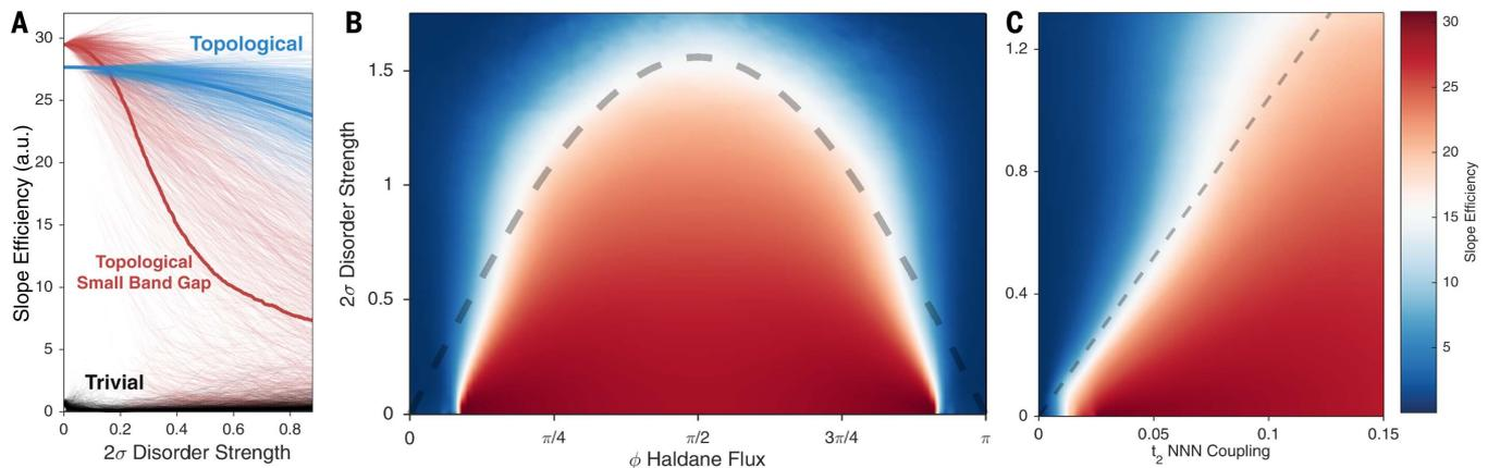
**Fig. 4. Slope efficiency versus disorder in the topological and trivial laser systems (Haldane model).**
