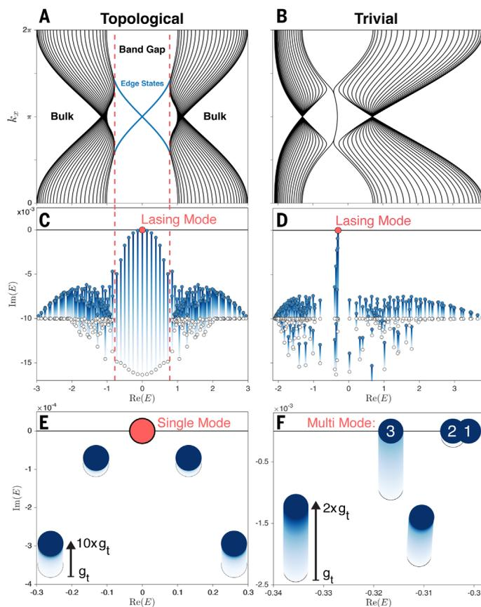
(a semi-infinite chain of resonators, which is what makes this an open system) and its coupling to the cavity. To promote lasing of the edge modes, the gain ( $g$ ) is provided only to the resonators on the perimeter (Fig. 1A). In general,  $g$  is a function of the frequency; however, in semiconductors the gain is broadband (relative to the inter-ring coupling constant), and hence it is assumed to be frequency-independent.
