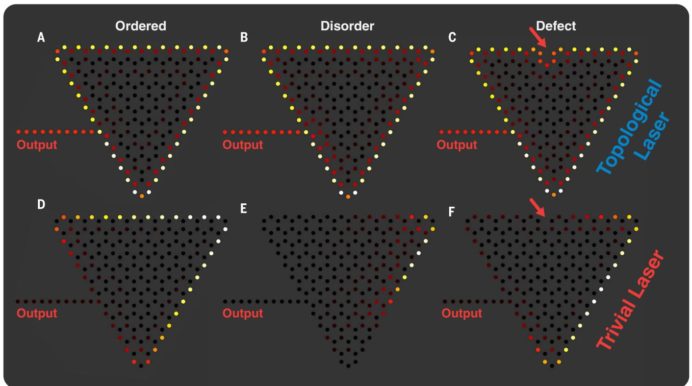
**Fig. 2. Lasing modes in the topological and trivial cavities (Haldane model).** (A to F) Steady-state lasing modes (colors indicate amplitude) for the topological and trivial cavities with no disorder [(A) and (D)], disorder [(B) and (E)], and a defect (a missing gain resonator at the perimeter) [(C) and (F)]. Being unidirectional and extended, with almost uniform intensity, the lasing mode in the topological cavity [(A) to (C)]
