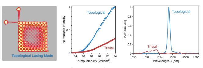
Left: Top-view photograph of the lasing pattern (topological edge mode) in a 10×10 array of topologically connected resonators, and the output ports. Center: Output intensity versus pump intensity for a topological-insulator laser and its corresponding trivial counterpart. The enhancement of the slope efficiency is approximately threefold. Right: Emission spectra from a topological-insulator laser and its topologically trivial counterpart.
