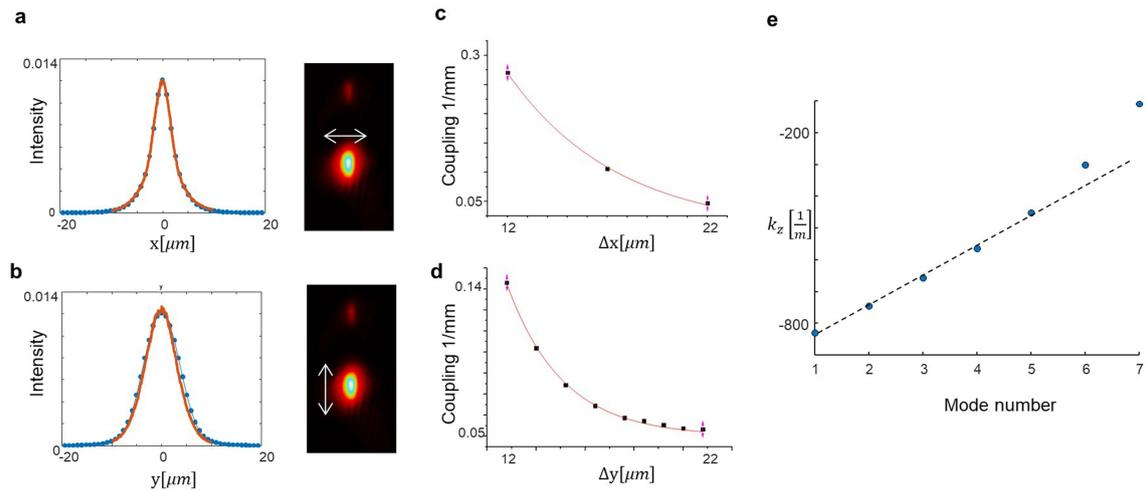
**Extended Data Fig. 8 | Stages in the preparation of the experimental model.** **a**, Horizontal cross-section of the intensity of a propagating mode of a single waveguide (orange line) and the cross-section of the mode in the simulations (blue line). The image on the right is the intensity distribution of the mode in the direction of the cross-section. **b**, Same as
