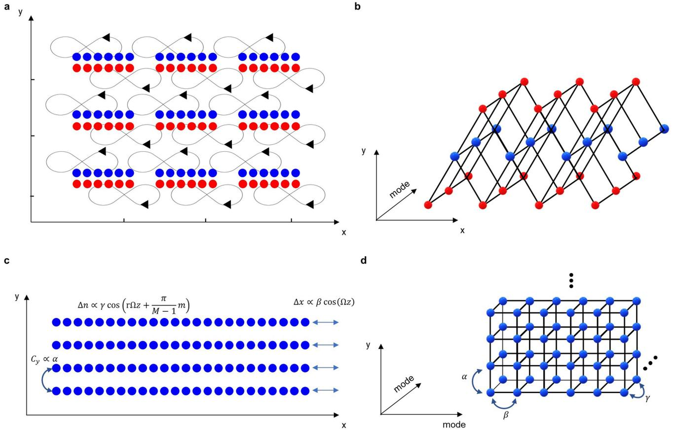
**Extended Data Fig. 1 | Increasing the dimensionality of a two-dimensional lattice of waveguides.** **a**, One-dimensional columns arranged in a two-dimensional lattice. The columns oscillate along the black paths in the direction indicated by the triangles. Red and blue colours indicate different columns in the same unit cell. **b**, Representation
