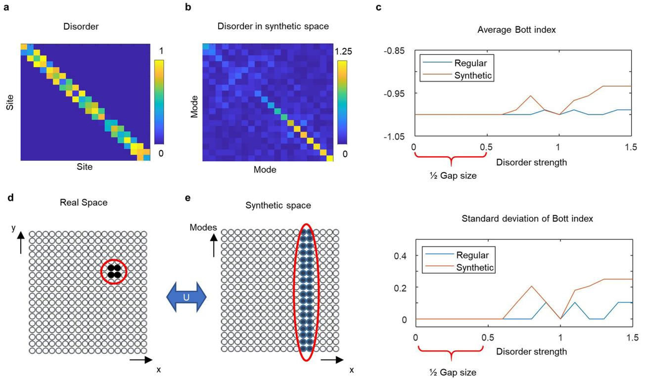
**Extended Data Fig. 5 | Disorder in synthetic space.** **a**, Typical disorder introduced to the Hamiltonian of a one-dimensional lattice. The Hamiltonian is in real-space matrix representation (the colour bar corresponds to the real part of the value of the matrix element). **b**, The disorder shown in **a** after transformation to synthetic space. **c**, Standard deviation and mean value of the Bott index averaged over 10 random
