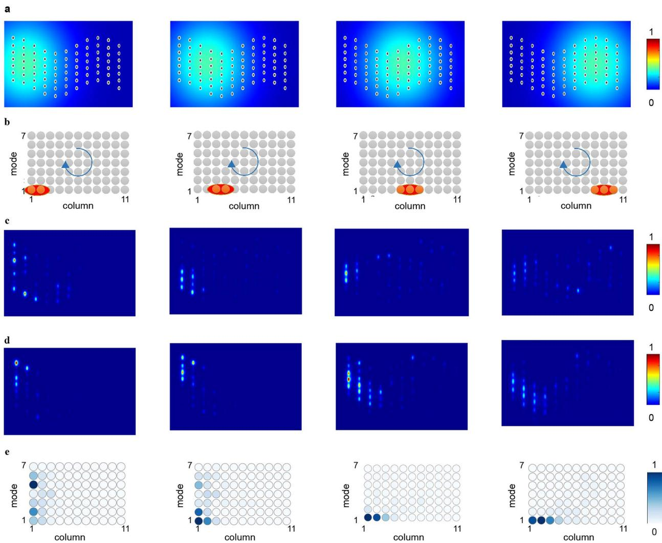
**Extended Data Fig. 7 | Experimental results for a sample fabricated with different parameters.** Illustration of an incident narrow Gaussian beam directed towards the input facet of a synthetic-space topological lattice fabricated with parameters different from those used in the experiments presented in the main text (here,  $\phi = \pi/4$ ,  $\Omega = 91 \text{ m}^{-1}$  and
