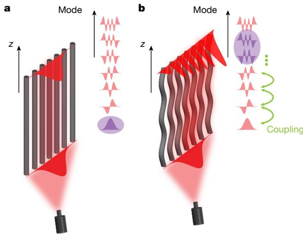
**Fig. 1 | Forming a one-dimensional lattice in a synthetic modal dimension.** **a**, One-dimensional lattice with a spectrum of  $N = 7$  eigenmodes with equally spaced propagation constants. **b**, Oscillating the lattice in the longitudinal direction causes each eigenmode (of the straight lattice) to couple to its nearest neighbours, forming a lattice of coupled modes.
