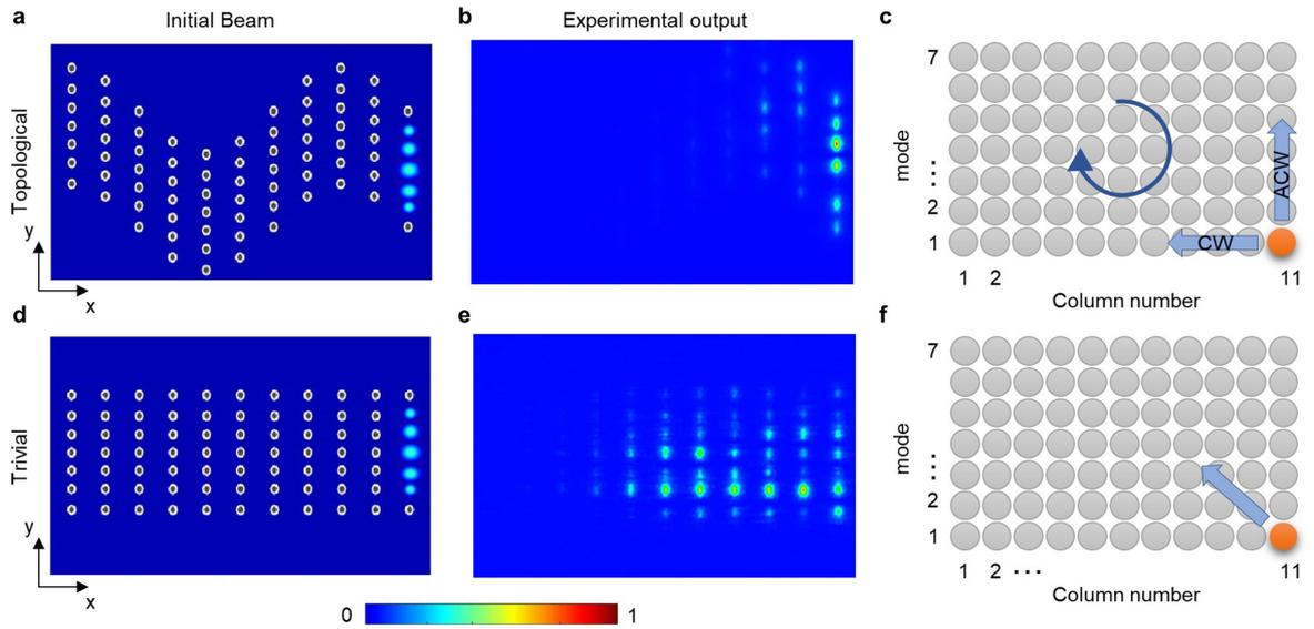
**Extended Data Fig. 6 | Exciting the anticlockwise edge state.** **a**, Initial excitation of the first mode in the rightmost column of the topological lattice. **b**, Output intensity (colour bar) corresponding to **a**. **c**, Direction of
