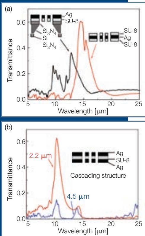
(a) The transmission spectra of the single metallic structure (black) and the symmetrical metallic structures (red), and the left inset is the schematic view of the stencil mask; (b) The transmission spectra of the cascaded metallic structure with the SU-8 thickness of 2.2  $\mu\text{m}$  (red) and 4.5  $\mu\text{m}$  (blue).
